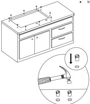
Insert anchors into drilled holes and lightly tap with a hammer until flush.
