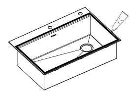
Use a bead of silicone (or preferred adhesive) around the rim of the sink. Check the alignment of the sink to the cutout in the countertop. Place sink over cutout hole and press firmly.
