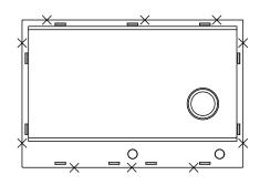
for mounting brackets. Mounting holes should be 1/2" from edge of sink.
