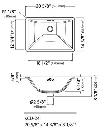
\*NOTE: Each sink may have a 3% dimension tolerance. Please measure the sink prior to installation.
