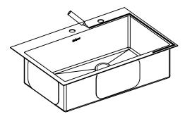
• Use a bead of silicone (or preferred adhesive) around the rim of the sink. Check the alignment of the sink to the cutout in the countertop. Place sink over cutout hole and press firmly.
