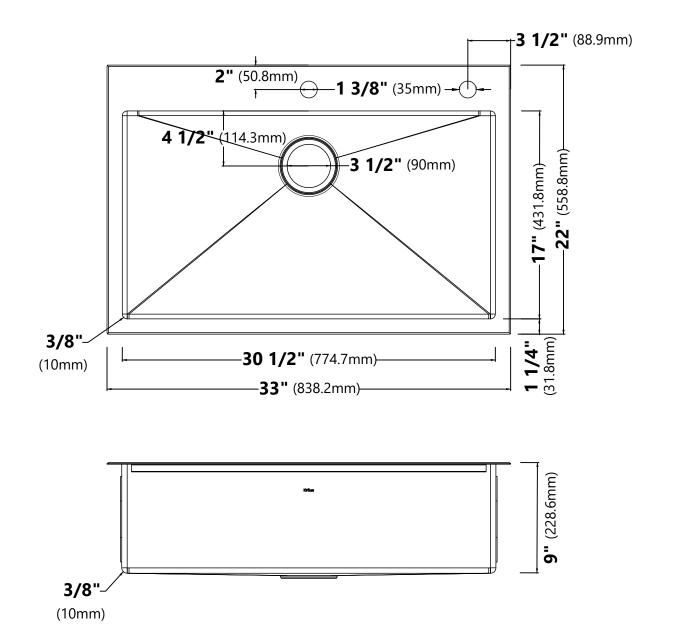
Model #: KHT400-33 Sink Dimensions: 33" x 22" x 9" Min Cabinet Size: 36" Matching Grid: KBG-T400-33 Drain Model #: ST-1
