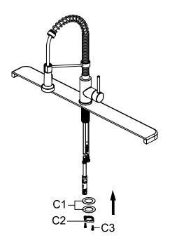
Install the rubber washer and metal washer (C1) onto the threaded mounting shank.
