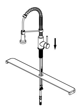
Optional No Escutcheon Installation. Insert faucet body through the hole in the sink.
