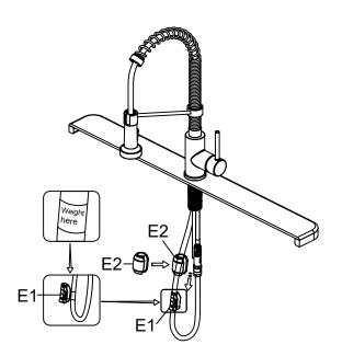
Install the weight clip (E1) at the point of the hose marking "weight here". Insert the weight (E2) onto the clip (E1) by sliding it down onto the clip (E1).
