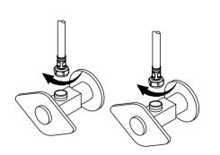
Attach waterlines to angle stops and tighten until snug. Turn on angle stops and check for leaks. (DO NOT TURN FAUCET ON)
