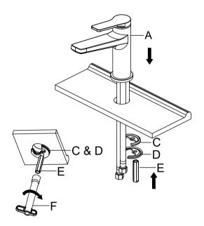
Place the faucet (A) through the mounting holes in the sink until the faucet (A) sits on top of the sink. Secure the faucet (A) to the sink using the rubber (C) and metal washers (D) and lock nut (E) provided. Ensure the washers (C&D) and waterlines have no interference.
