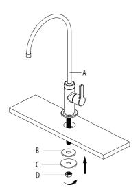
Place the faucet assembly (A) through the selected hole in the sink or countertop. On the underside of the sink or countertop, slide the rubber washer (B) and metal washer (C) onto the stud. Thread the mounting nut (D) onto the stud, and tighten securely using your wrench.
