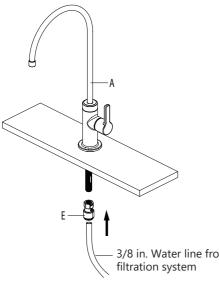
Thread the quick connect adaptor (E) onto the end of the faucet assembly (A) stud, and tighten securely using a wrench. Connect the 3/8 in. water line from the filtration system by pushing the line into the connector (E). Pull down on the 3/8 in. line slightly to ensure the quick connect fitting has engaged.
